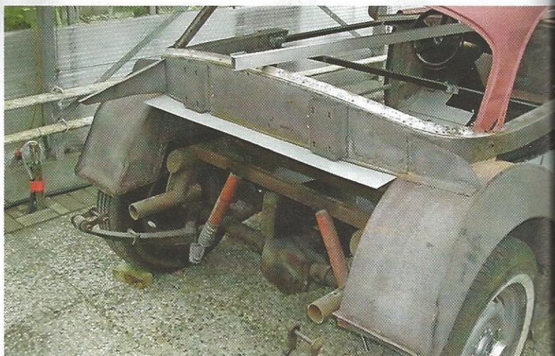
Lopping off the entire rear end might seem drastic, but it's necessary when there's nothing solid underneath
