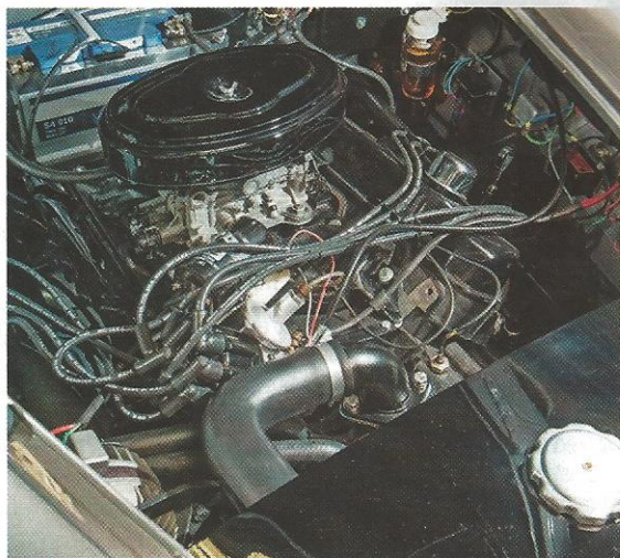
Single four-barrel carburettor is standard on all automatic transmission HKs
