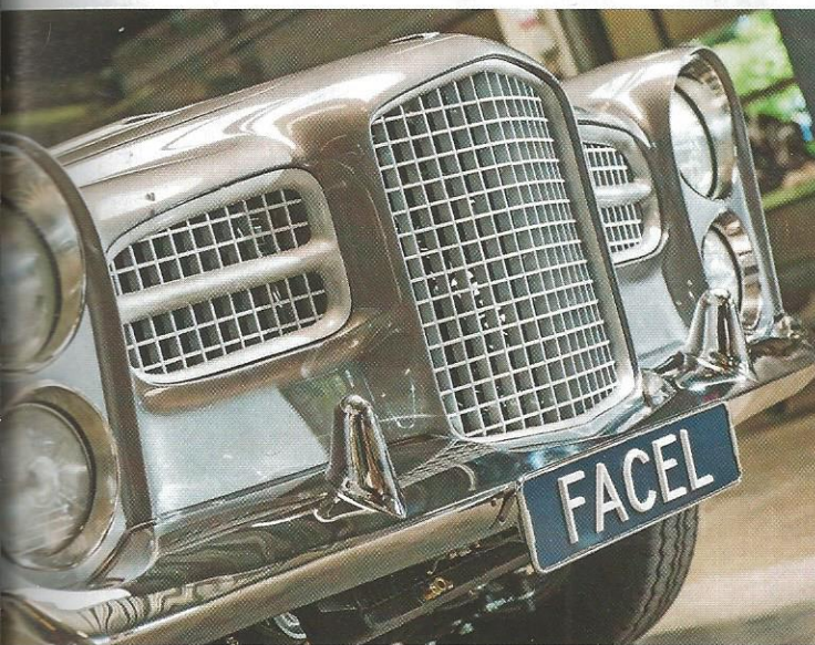
The new nose section was formed using a CNC tool to press sheet steel on to the wooden buck
