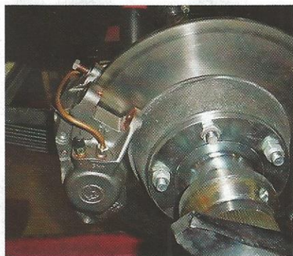
Upgraded rear brake system with Girling calipers
