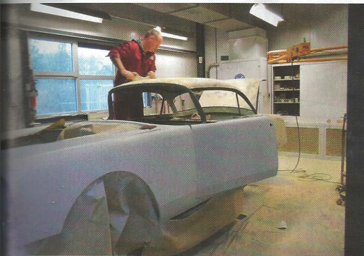
...complex body to this stage involved epoxy primer, two different grades of spray filler and a coat of primer
