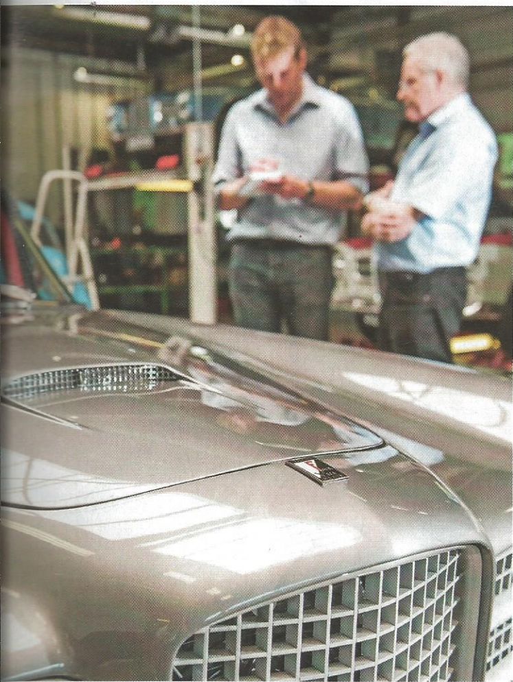
...finish is a painstaking recreation of the HK500's original Glasurit colour sampled from the old paint
