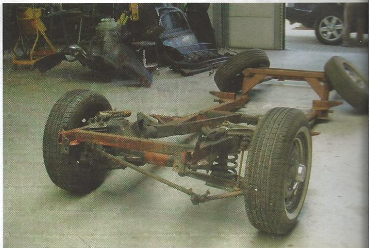
Chassis and body were separated for long periods of the restoration to allow work to progress in parallel
