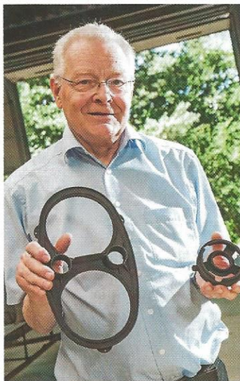
3D-printed light bracket and steering boss
